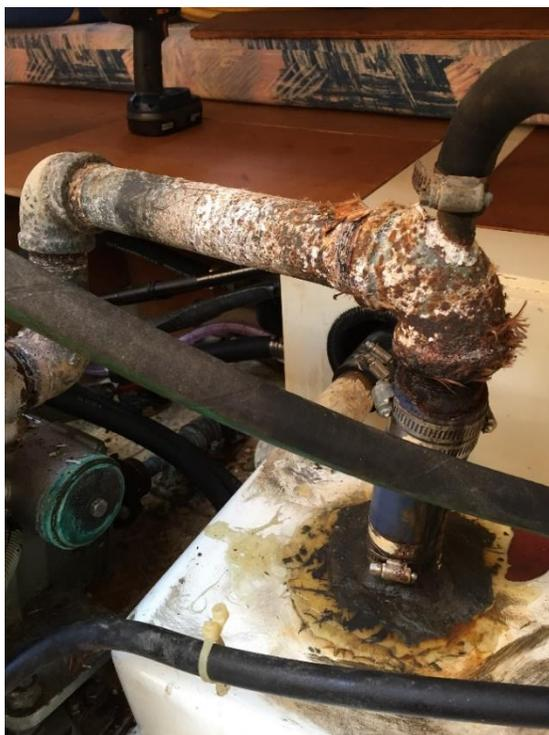
Original muffler and manifold exhaust riser after removing the thermal wrap
