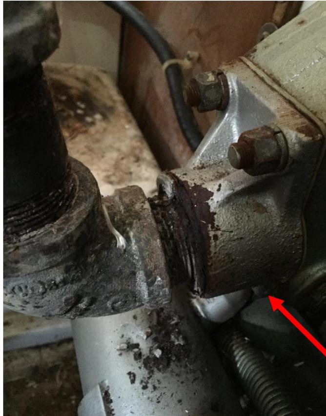
The third nut is located on the bottom of the flange.
