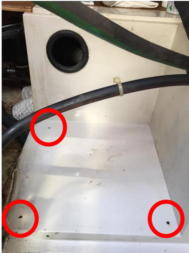
3. After setting the new muffler in place, I marked and drilled the new mounting holes in the muffler tabs and boat mounting location. I used four #10, 1 1/2" stainless steel machine screws and washers.
