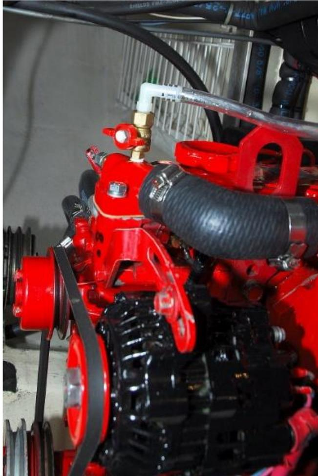
I designed this a number of years ago and have installed one on every engine since. The M-25 has a spot for a real ball valve on top of the t-stat housing.
