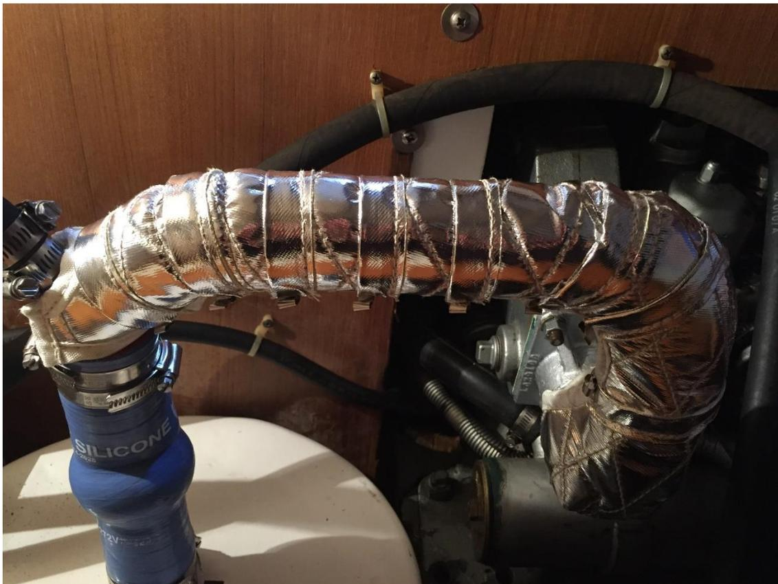
Thermal jacket cover installation from the back
