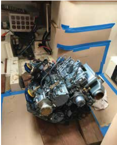
With the small plywood bulkhead between the galley and aft cabin removed, access to the engine is easy.
