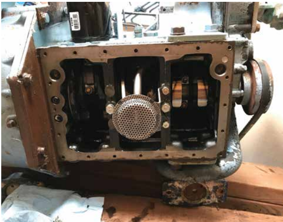
With the oil pan removed, I inspected the bottom end of the engine - it looked very clean.
