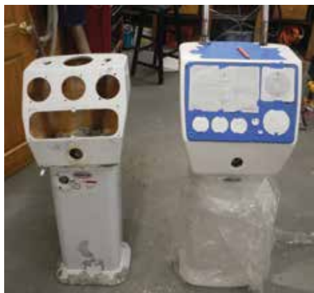
Fig 3. Original and new Edson Vision NV pedestal side by side. New pedestal head is a few inches wider and taller. Face plate was taped out and templates assembled before cutting faceplate.
