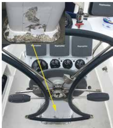
Fig 1. Original pedestal stand with debonding paint.
