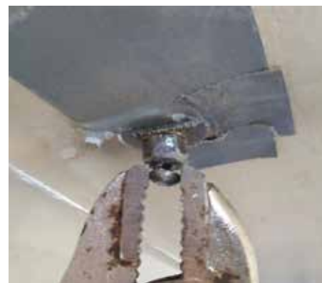
Removing acorn head crown after Dremel cut
