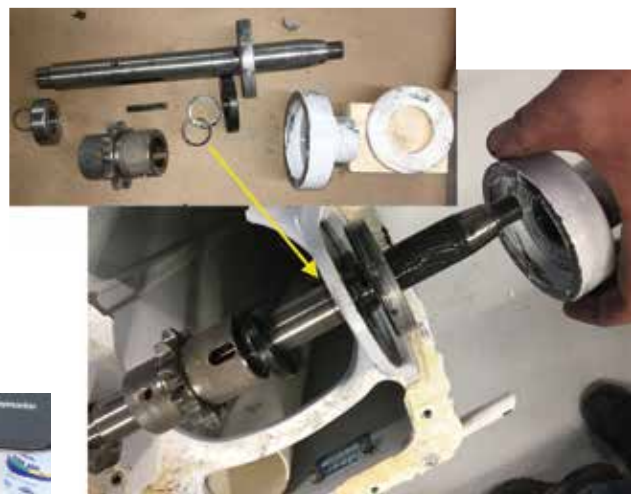
Fig 2. Top image shows steering gear assembly laid out in order of placement in pedestal. Lower image shows assembly as it was being disassembled, arrow points to where one of the spring retaining rings was. Other was on back of shaft holding bearing in place.
