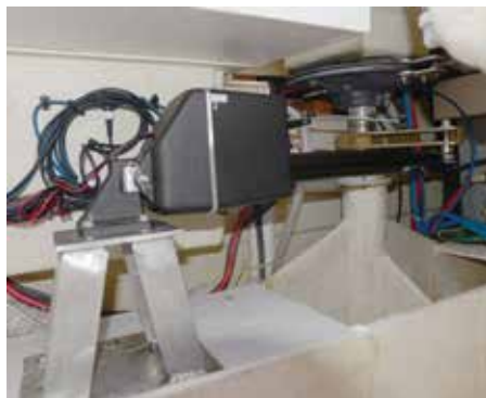
Fig. 8 : Image from aft lazarette crawl space shows Raymarine Type 1 mechanical linear drive on fabricated aluminum stand. Drive unit is connected to Edson tiller arm which in turn is attached to rudder shaft.
