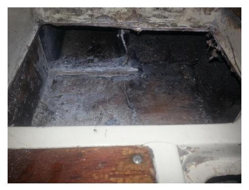
Then I made the mistake of probing a bit at the lower timbers - and the 'fiberglass' layer on top popped right off. It appears to be what my boatbuilder friend calls "bear shit" - leftover polyester resin thickened with leftover sawdust, and often used in boat building to fill gaps. This chipped right off and the timber underneath were exposed.
