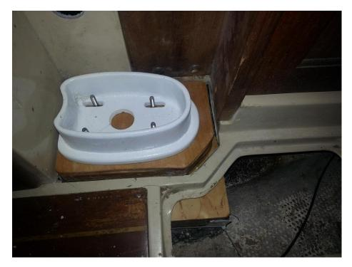
The final step of the day was bore four 5/8" holes down into the stack, fill them with epoxy, and stick 5/16 bolts into them upside down. These will form the studs to mount the mast step itself, and doing it this way I hope to prevent water travelling down the studs and into the wood, which as mentioned I think caused a lot of my problem to begin with.
