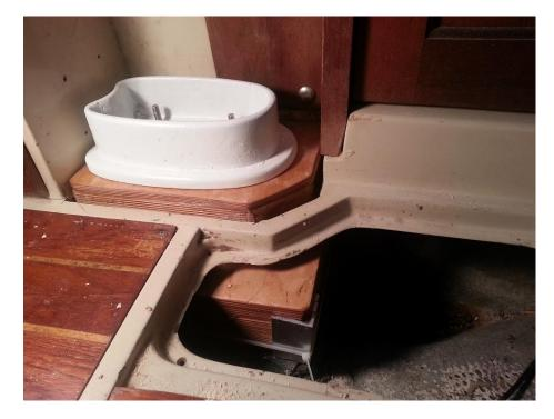
The top of the stack comes right through the floor and I will not be attaching them together, I don't believe the floor adds much strength to the system and I do believe the floor/hull clearances are prone to moving, this way I don't anticipate any new cracks being formed.
