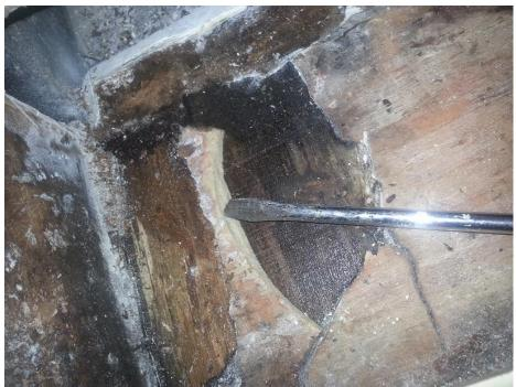
What I found is three very thick hardwood beams spanning the keel box and bedded in polyester goop. These were wet also, I would assume they wick water up from the bilge if there is more than 1/2" of water in the bilge. However they did not seem rotten except for one soft spot in one corner which I removed. I called a couple guys who would
