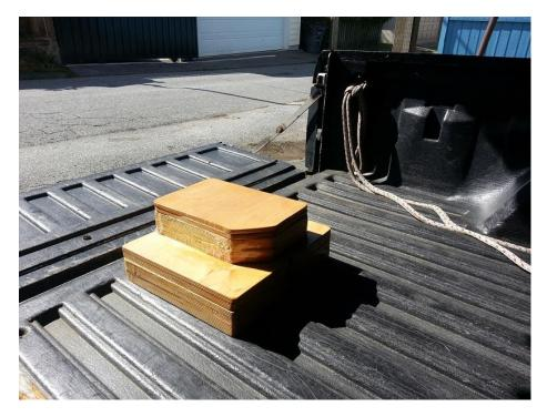
The whole mess was put together by sliding each layer into the bilge, coating the mating surfaces in epoxy, and sliding them together, then doing the same with the next layer and then screwing them down onto each other. The screws were buried in epoxy and always placed so that the piece going on top would hide the heads anyways. I don't expect to get any water into the wood.
