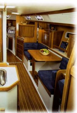
The two seats and game table to starboard can be made into a settee or berth with the cushions provided. The entertainment center cabinet can be fitted with a stereo and concealed TV. All interior teak has the warmth and durability only obtained with multiple coats of varnish.
