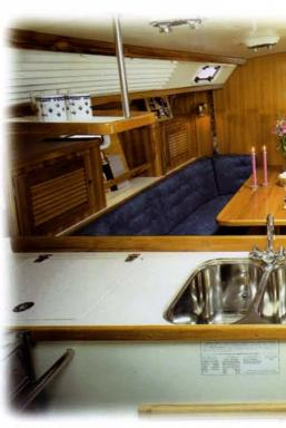
The galley is a functional 'U' shape, with composite counter tops and sinks that are near the centerline for proper drainage underway. The large refrigerated ice box is aft and a dry food locker is forward. A gimbaled, stainless steel LPG stove with oven is standard equipment.
