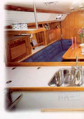
The galley and main cabin have received special attention to design and detail. The galley is a functional 'U' shape, with composite counter tops, sinks are near centerline for proper drainage underway. A large refrigerated ice box is aft and a dry food locker is forward. A gimbaled, stainless steel LPG stove with oven is standard equipment.
