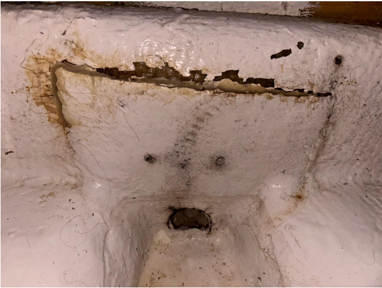
The next picture is more directly overhead and captures the extent of the bulge where the glass is being forced away from the stringer. Bilge hose is no longer attached to the damaged area.
