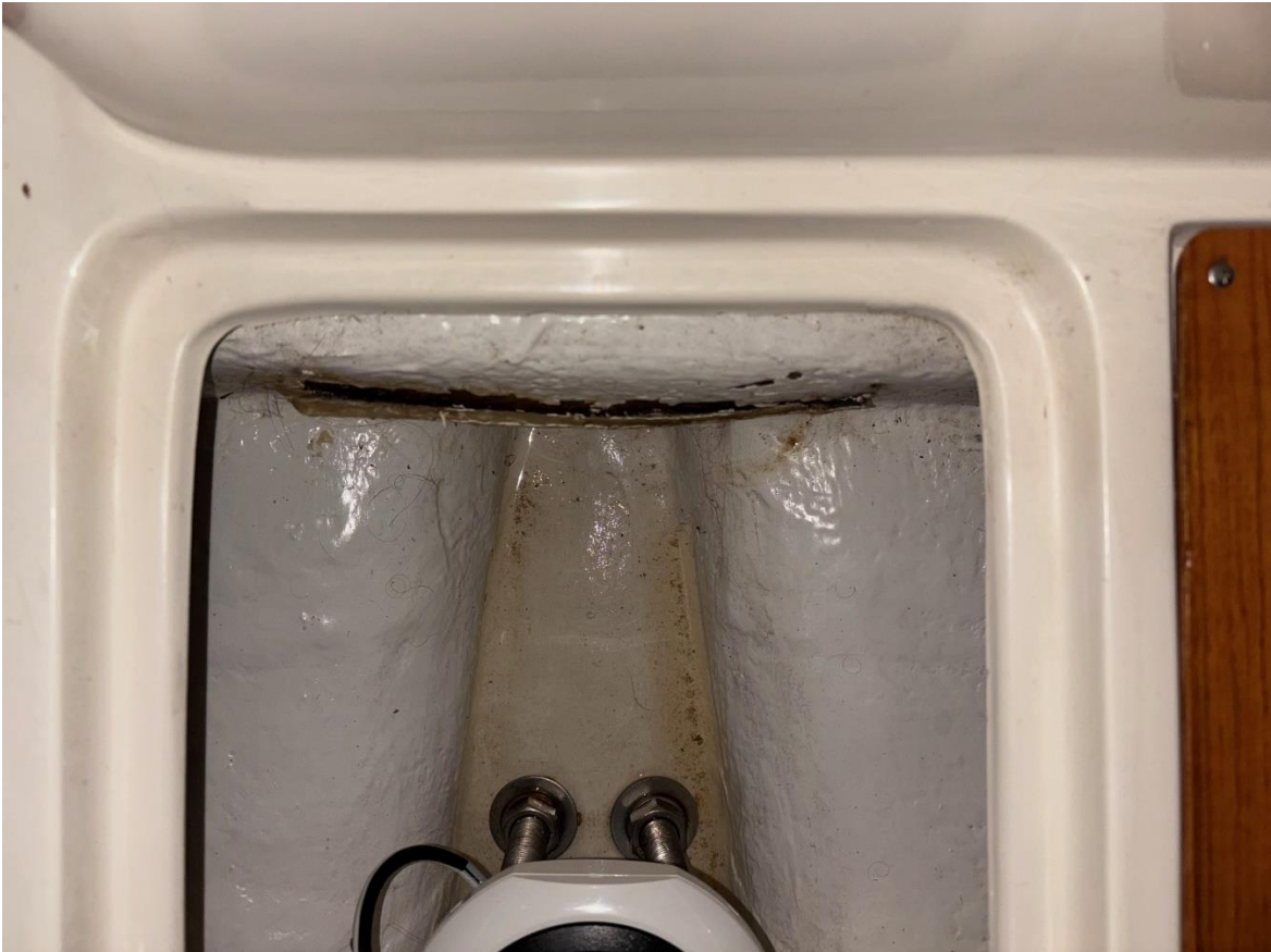
The next picture is more directly overhead and captures the extent of the bulge where the glass is being forced away from the stringer. Bilge hose is no longer attached to the damaged area.
