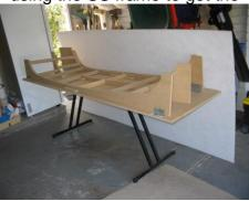
Core material seen standing upright behind the mold. I tested the mold by placing the SS frame on the mold to verify tolerances as I had to allow 15mm for the thickness of the FG top.
