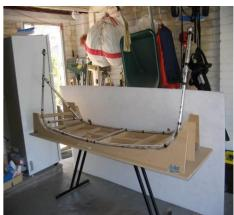
Nidaplast is a very light material which looks like a honeycomb covered both sides with a light FG material. I laid the material on the floor, weighing down template and then cut using a sharp knife.
