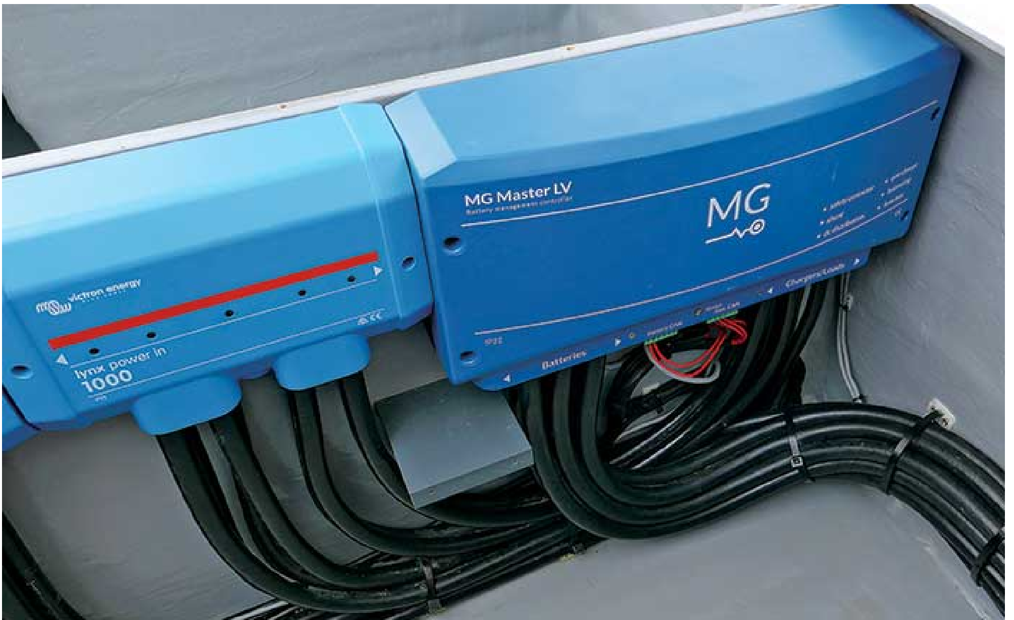
A remotely mounted battery management system (BMS). This is allowed under ABYC standards, however, installers must ensure that nothing is powered directly from the battery(s) before the BMS.
