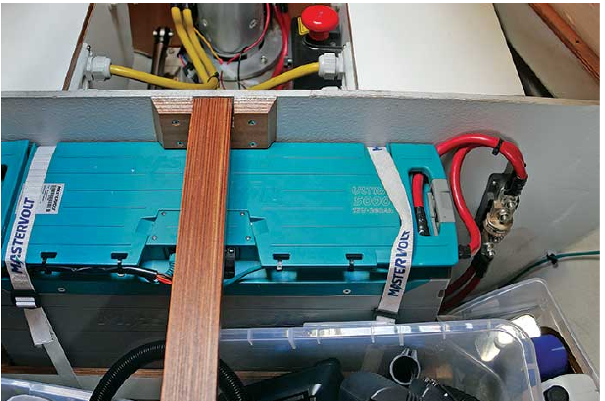
A Mastervolt Li-ion battery with integrated BMS and the standards-required class "T" fuse to its right mounted on the bulkhead. This is an additional expense when upgrading to Li-ion batteries.
