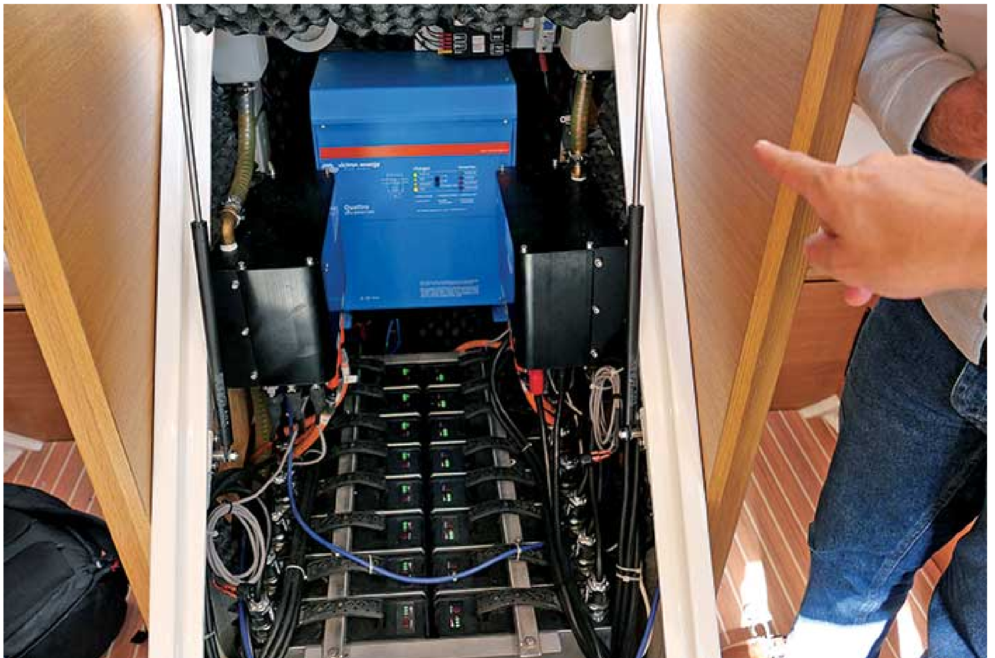
Large bank of li-ion batteries with a properly programmed charger (blue box) used to supply an e-powered boat using twin Oceanvolt electric drives.
