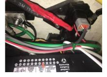
Everything went very smooth after that. I used 2 each #8 x ¾ stainless screws to fasten both the shunt and the smart shunt to the bulkhead. You might notice on the battery side of the smart shunt I have two wires attached to the nut. For my house bank I have 4 GC2 FLA batteries, two in the location shown and two under the nav seat.
