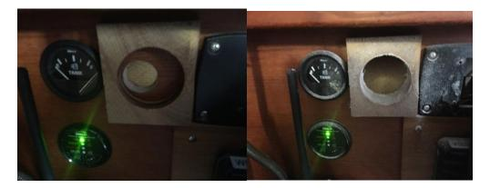
Here you can see I'm getting ready to pull the wires from the battery compartment to the panel. First I push the end without the connector from the battery compartment to an area directly below the gauge (one bulkhead aft). Then I need to get the wire from floor level to behind the panel. I really like the 6'
