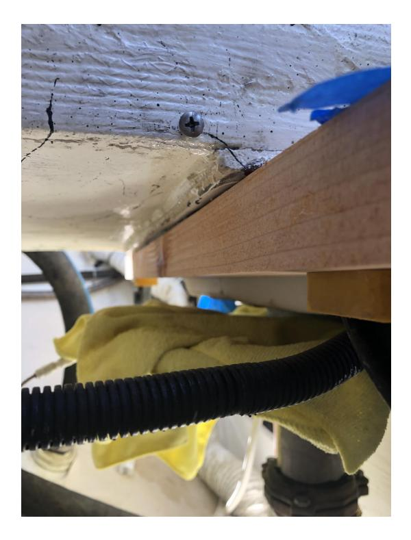
Caul in place after epoxy injected (view from starboard lazerette). Note rags on radial to catch run out of epoxy. Runout has been clean up at this point, Gorilla tape on caul for release in case it ended up glued to the fiberglass.
