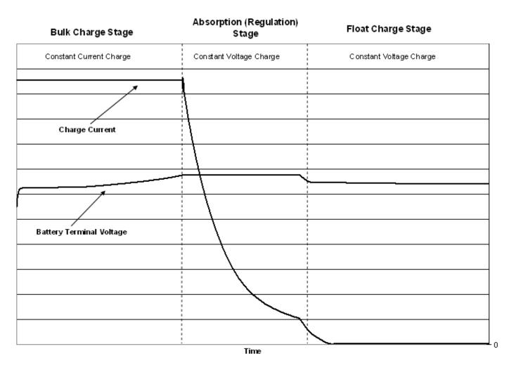
**Bulk Charge Stage** – Current is applied to the batteries at the maximum safe rate they will accept until voltage rises to near (80-90%) full charge level. The battery voltage rises because the charging current that is provided by the battery charger is replenishing its internal charge capacity. The charger current is flat (constant) and the battery voltage is rising.
