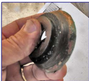
Heavy corrosion on clutch cones
