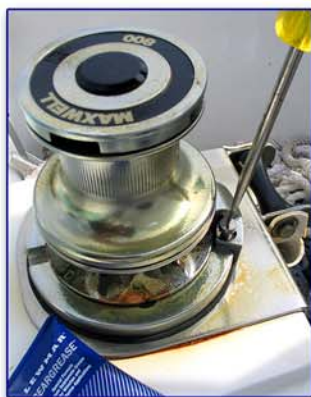
Windlass base prior to re-assembly - grease shaft & threads.
