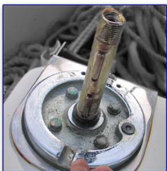
Windlass base prior to re-assembly - grease shaft & threads.
