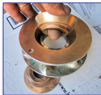
Clutch assembly after cleaning with solvent & wire brush. I applied "Lewmar Greargrease" (or see Maxwell specs) to clutch surfaces.
