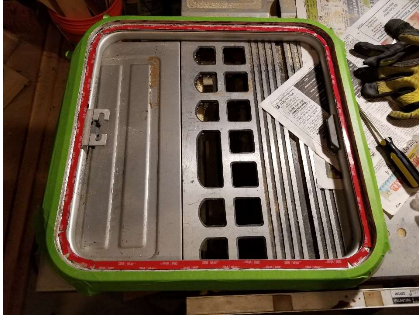
The old lens is out, the VHB tape is down in the frame (red backing), and the green masking tape is one the frame.
