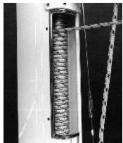
The swivel block 's upper part is fitted to the mainsail halyard and its lower side receives the mainsail. The swivel block acts as guide for the furling rod in the upper section. It is possible to remove it from the furling mast for maintenance purposes.
