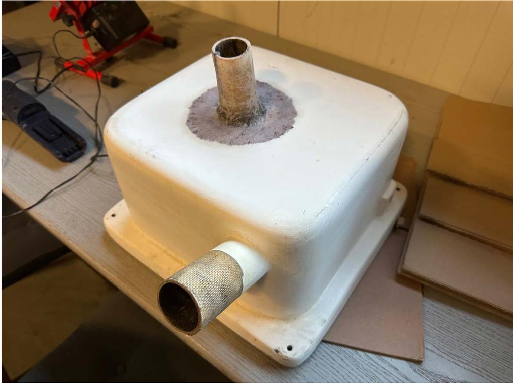
Inlet pipe repaired with additional layer of GRP.
