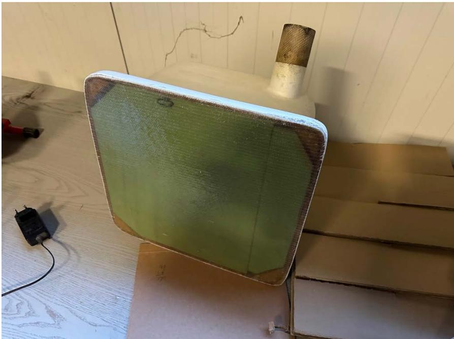
Bottom part fully filled with epoxy till flush.
