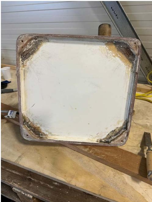
At the bottom bad connections and signs of earlier repairs by previous owner.
