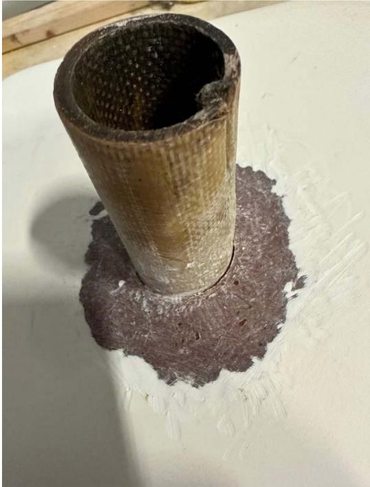
After proper cleaning inlet of the muffler a visible bad connection to the housing and crack in the pipe itself.
