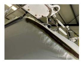
After "opening" the joint and proper cleaning we reinforced the whole transom with epoxy and layer of glass.
