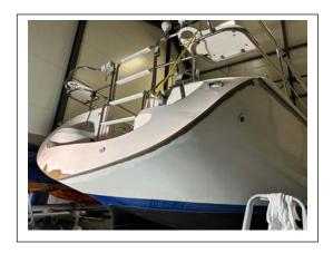
As can be seen on the pictures we removed also all the hull striping / ships name etc. Of course, there were also other small damages / scratches to the hull which could be attacked also during this repair.
