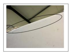
First, we started to grind-off all the gelcoat of the transom.
