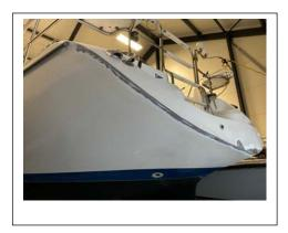
Having the gelcoat grinded off, we were able to conclude what the cause was of the hair-cracks in the gelcoat.
