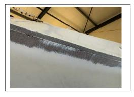
The joint between the hull section and the deck/transom section is clearly visible after grinding off the gelcoat layer.
