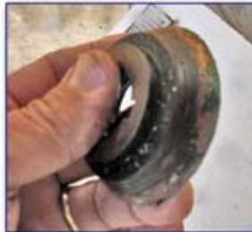
Heavy corrosion on clutch cones
