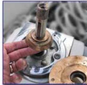
Re-assemble 3 pc brass clutch on shaft over 2 keys
