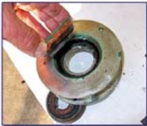
Remove clutch assembly off shaft. Brass cones may need to be pushed out by screwdriver if stuck (mine were). Note heavy corrosion.
