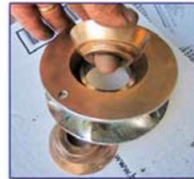
Clutch assembly after cleaning with solvent & wire brush. I applied "Lewmar Greargrease" (or see Maxwell specs) to clutch surfaces.
